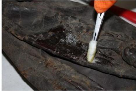
**Photo 10. Softening tests for a water sack.**
