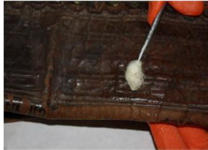
**Photo 6. Softening tests for the girdle**
